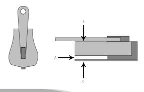
The most common reason why zips burst open is that the zip slider does not close the coil tightly enough. Wear and tear may cause the gap marked A to open up.
