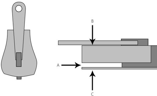
The most common reason why zips burst open is that the zip slider does not close the coil tightly enough. Wear and tear may cause the gap marked A to open up.
